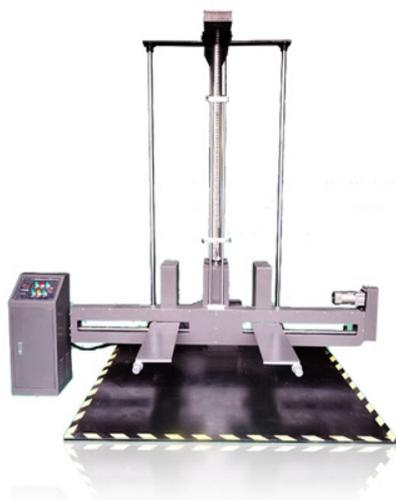
This series drop test bench for measuring the main simulation packages in the transportation, loading and unloading process under drop impact influence, identification package impact strength and packaging design.
